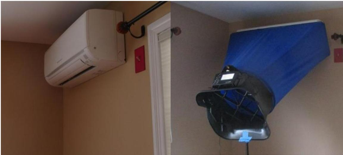
**Figure 3.** DHP Supply Airflow Spot Measurement
